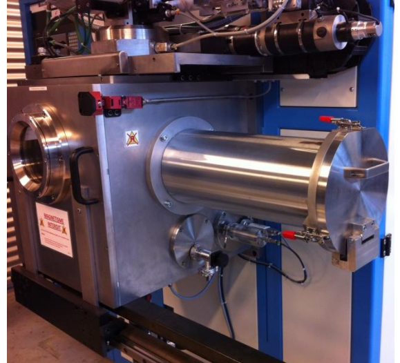
Chamber's tubular extension : Ø200 mm x 500 mm
